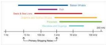
The audible range of hearing for marine fauna spans from five Hz up to about 200 kHz. A propeller-driven ship has a number of noise sources: the main and auxiliary engines, electric motors and the flow noise due to turbulence in the boundary layer and the wake of the hull and appendages.
